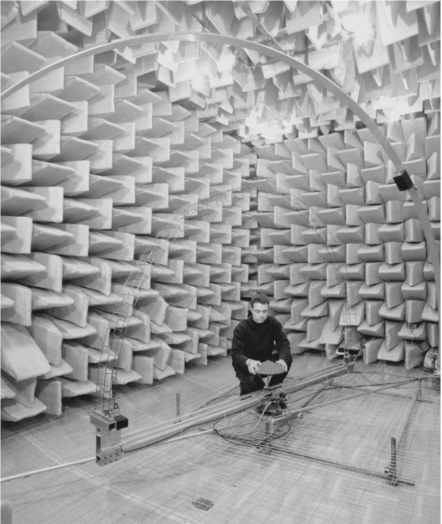
Figure 12.2. Typical anechoic room. (Courtesy Salford University.)
