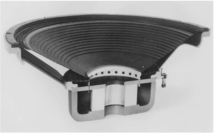
Figure 11.33. Cutaway view of 380 mm bass musical instrument loudspeaker with 100 mm diameter voice-coil and centrally placed Alnico magnet. (D140, Courtesy JBL Inc.)
