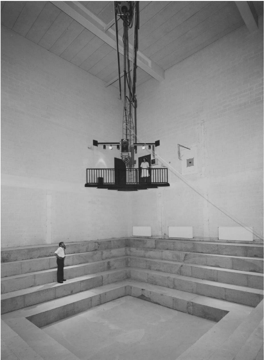
Figure 12.3. Reverberant room measuring 12\text{ m}^3 . (Courtesy Bang and Olufsen.)
