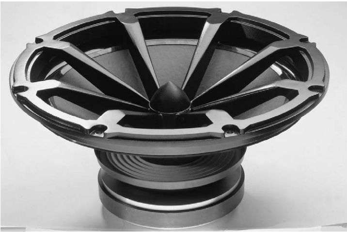
Figure 2.29. In this high-power woofer, dissipation is aided by an aluminium chassis which is outside the enclosure. (Courtesy Volt Loudspeakers Ltd.)
