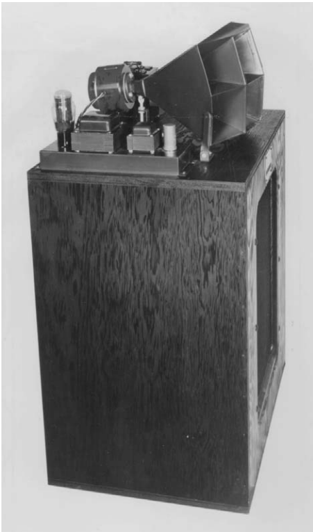
Figure 11.3. Lansing 'Iconic' two-way system of the late 1930's, with field-coil energized transducers. (Courtesy of JBL Inc.)
