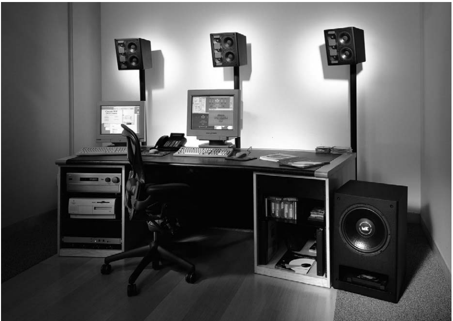
Figure 11.23. Multi-channel 5.1 surround sound monitoring workstation environment, showing left-centre-right front speakers and subwoofer. Not visible are left and right rear-channel surround loudspeakers. (MPS Series, Courtesy M&K Professional.)
